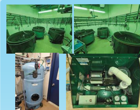
Figure 2. Photos of experimental settings. Control room (top left) with oxygen injection vessel (bottom left), and test room (top right) with nanobubble generator (bottom right)
